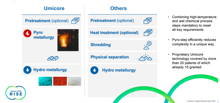
Fig 17. Umicore's recycling method (hybrid recycling model combining pyrometallurgy and hydrometallurgy) compared to others recyclers' method.
